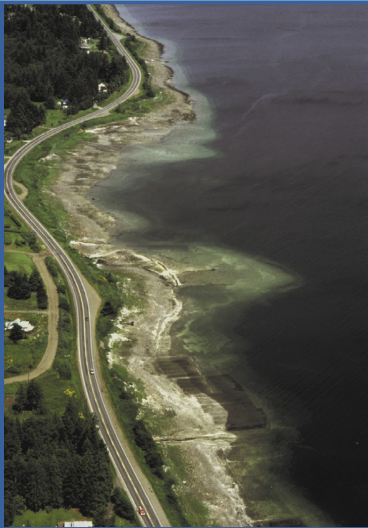
Historic settlement patterns frequently include roads adjacent to eroding shore areas. Expensive shore protection measures are often required where roads have been widened to meet modern safety standards, or to accommodate more traffic.
