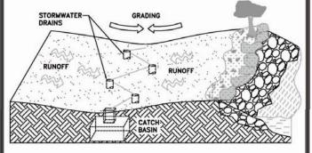
Storm water runoff can flush accumulated oils and pollutants from upland surfaces into nearby bodies of water. Pollution from multiple sources, known as non-point source pollution, can be managed through site planning that incorporates catchment, interception, and containment of run-off.
