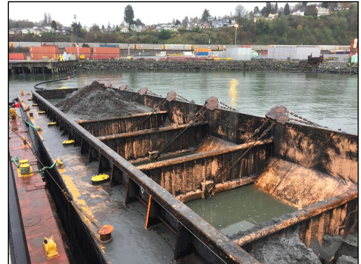
Bottom dumping barge typically used to transport clean material to an open water disposal site
